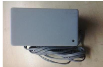
**Description:** Telenet's Midspan POE is a Power-over-Ethernet (Poe) power supply which provides DC power for one Poe-equipped device by "Injecting" DC power through the Spare Pair of the CAT5 (10/100Mbps) Ethernet cable
